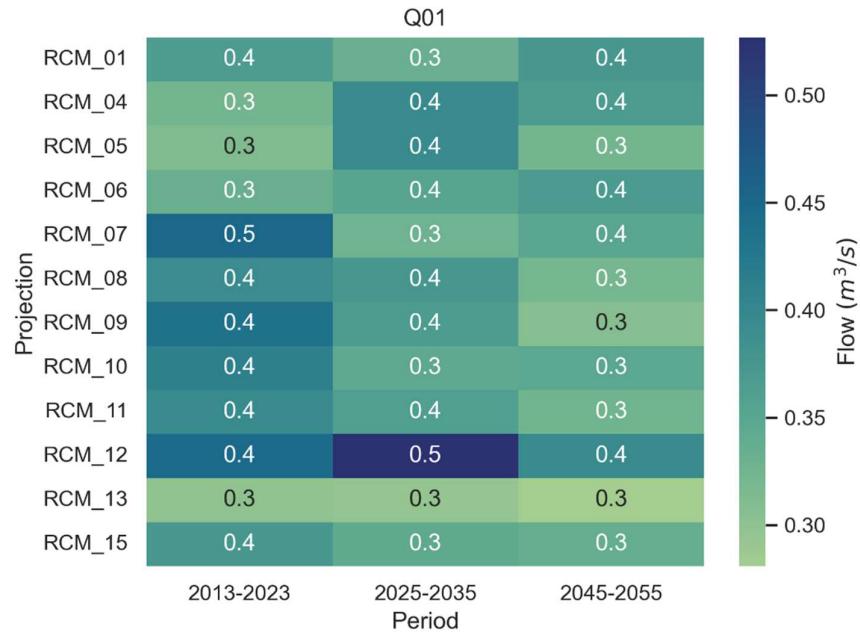
Figure 7-59 – Heatmap showing the 1 th percentile flow for different periods from 2013 to 2055 for each ensemble member in the eFLaG dataset
